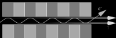
Wiggler: Intensity I \sim N continuous spectrum
