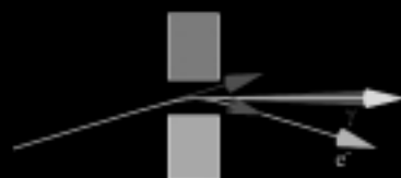
Bending Magnet: Intensity I \sim I continuous spectrum
